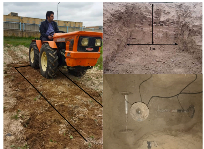
Fig. 1. Goldoni tractor moves over the soil surface (left), a scheme of digged soil profile after the tractor pass (Right top) Placement of strain transducers including endplates inside soil profile in longitudinal, lateral and vertical directions.
